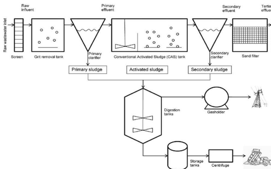
**Figure 1: Typical wastewater treatment plant processes with sand filtration as an example of tertiary treatment (Source Berthod et al., 2016).**
